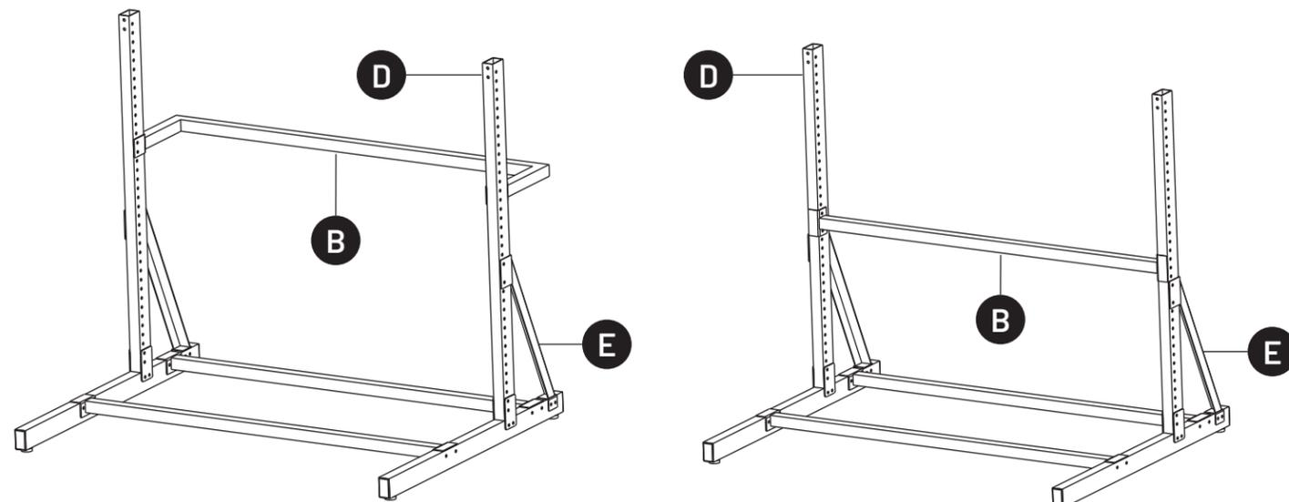
U-Shaped Bar: We recommend starting with 6 holes between the Diagonal Brace (E) and the Horizontal Support (B). Adjust as needed to align with the rear tires of your bikes.
