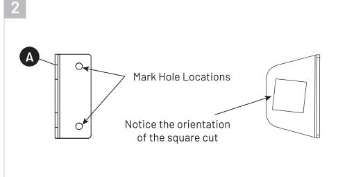
Align the mounting holes on the left Wall Bracket (A) with the previously marked wall stud. Make sure it is at a desired height and use a level to ensure the mounting holes are straight up and down.
