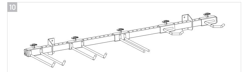
Continue to add attachments as desired. Keep in mind the spacing needed for hanging specific tools
