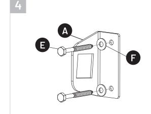
Mount the Wall Bracket (A) to the wall using the provided Wall Mount Screws (E) and Washers (F).
