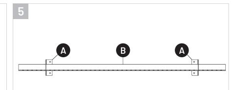
Slide the right Wall Bracket (A) onto the Horizontal Track (B). Then slide the Horizontal Track (B) into the mounted Wall Bracket (A). Align the mounting holes of the right Wall Bracket (A) with the second marked stud.
